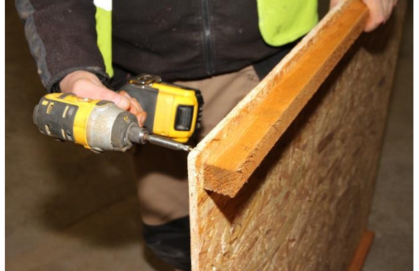
20. Attach Part H to Part J leaving the sheet overhanging 14mm at end of baton and equally spaced either end. Fix together using 4no 40mm screws. Repeat on second panel.
