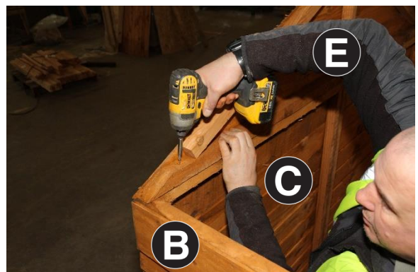
16. Fix Part E to Part C using 1no 60mm Screw. Repeat both sides.
