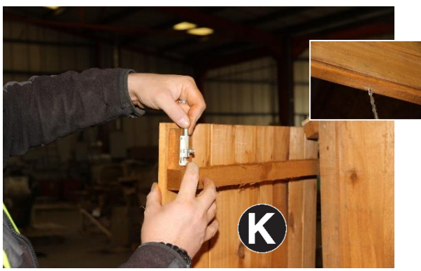
35. Attach slide bolt us 4no 25mm screws as above image. Close left hand side door align slide bolt mark and drill 8mm hole
